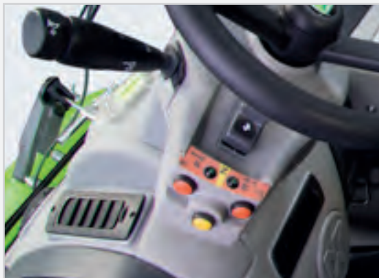
Dual-Shuttle reverse shuttle buttons
