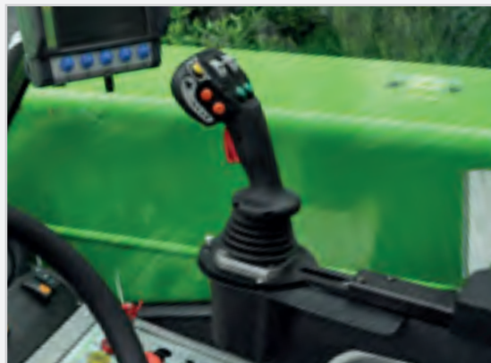
Armrest and Joystick with reverse shuttle
